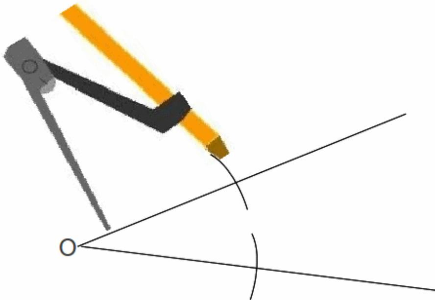
From each point where an arcs just drawn cross a line construct other arcs to cross as shown.
