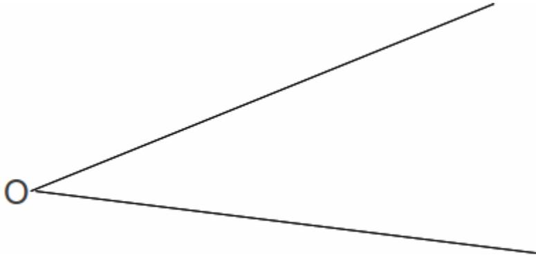
Put the point of the compass at O and draw arcs that cross both lines that constitute the angle.
