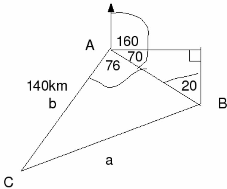
We draw a right angled triangle between A and B. Construct a right angled triangle at A and a horizontal line starting from A to the right. The internal angles of the right angled triangle are 70 and 20 degrees. Hence the bearing of A from B is  $360-20=340$  degrees.
