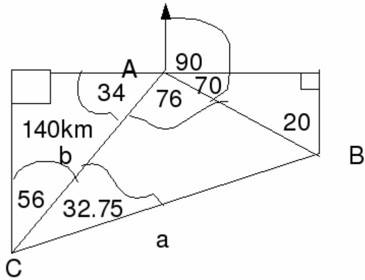
Construct the right angled triangle as shown, with the angles at  $C$  then the bearing is  $56+32.75=88.75$  degrees.
